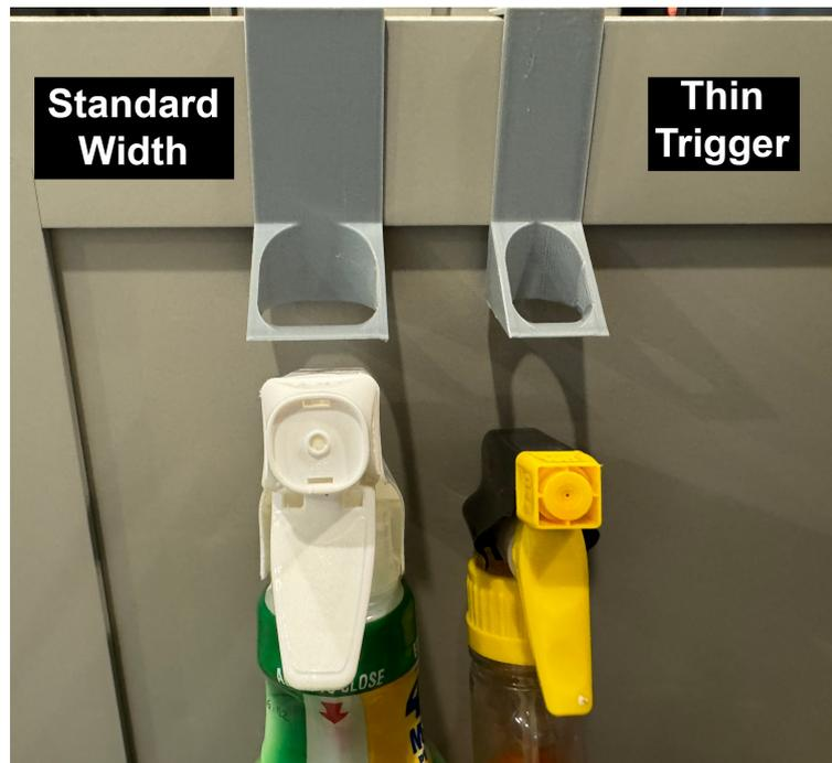
If you aren't concerned with how much of the bracket is visible from outside the cabinet, you can use the "**LongBracket**" variant, which might be sturdier/harder to knock off. This extends the visible exterior bracket from 5mm tall to 20mm.
