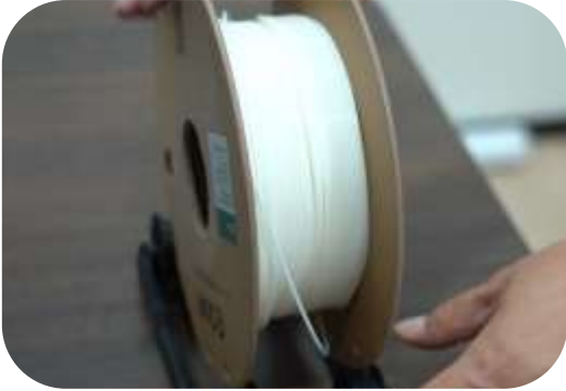
1. Place filament on spool holder
