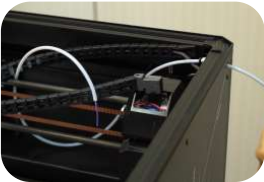
3. Until it passes through the PTFE tube and reaches the other end to ensure smooth delivery
