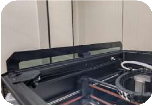
4. Hang the top glass cover plate on the left side of the printer
